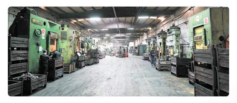
MSK FORGE combines its experience with technology and is able to produce parts of various sizes and types from 0.2 kg to 30 kg in its forging workshop using automated mechanical presses and hammer presses.
